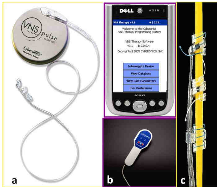
Figure 1a - Implanted components of the VNS system. 1b. Programming system components. 1c. The electrodes of the VNS system
